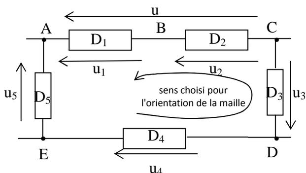
$$u_{AC} = V_A - V_C = V_A - V_B + (V_B - V_C) = u_{AB} + u_{BC}$$
